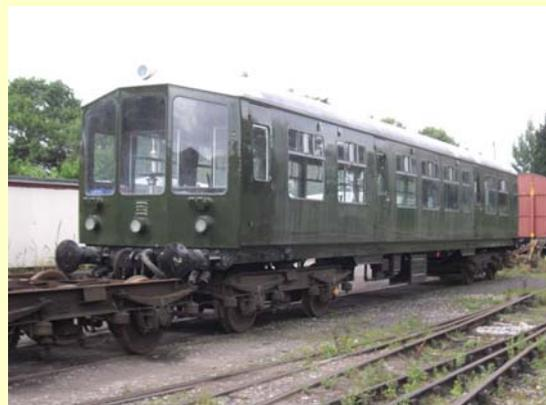
Guard's van of this vehicle progressing too, with the correct type of doors in the process of being fitted to the driver's side. The driver's side of the roof has been wire brushed ready for painting.
