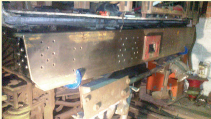
The new bufferbeam being trail fitted to 53645, 21/2/13 (M.Russell)
