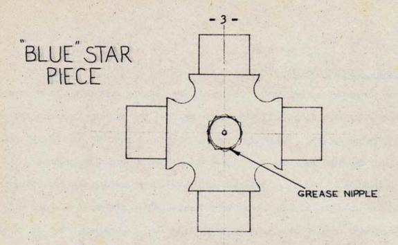
All the star pieces used up to now are fitted in needle roller bearings, but as the bearings have been known to give trouble, they are going to be changed to plain bushes. These star pieces will still be painted blue, so you will not know which type of bearing is fitted. However, it doesn't matter, because both star piece assemblies will be completely interchangeable.
