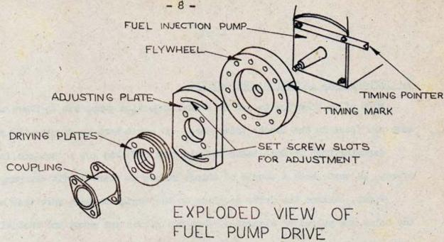
Connect up the drive coupling and tighten up. To do this you may find that you will have to move the pump flywheel slightly so that the marks are out of line. If so, slacken the set screws on the pump coupling adjusting plate, turn the flywheel so that the mank lines up with the pointer again, and re-tighten the set screws. Couple up and tighten the fuel pipe, and then tighten up the pump mounting bolts.
