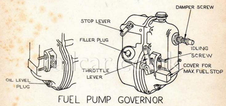
The next job is the governor damper. Remember, this is NOT the means of adjusting engine idling speed, and must not be used as such. On the end of the damper screw is a spring loaded plunger which bears on the end of the injection pump rack to stabilise it at idling speed and stop the engine hunting.
