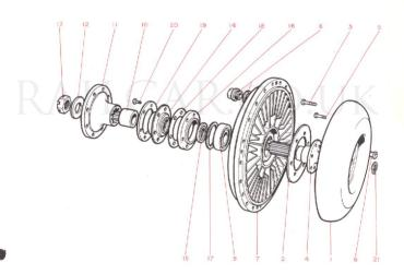
Fig. 3. Exploded view of fluid coupling (L - type).
