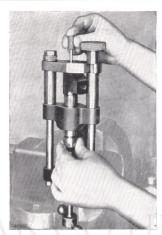
Fig. 68. Bouncing the needle valve on its seat.
