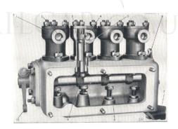
Fig. 48. Throttle motor showing cut-away view of operating piston.
