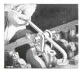
Fig. 49. Removal of bearing caps.
