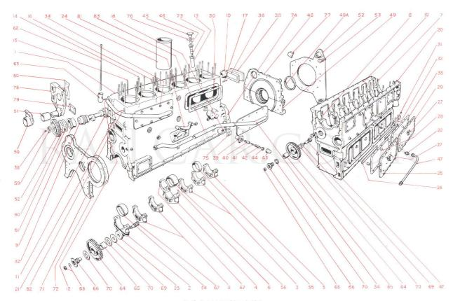
Fig. 37. Exploded view of the engine block.
