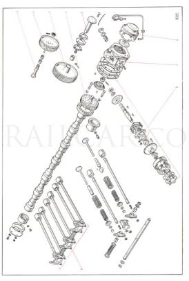
Fig. 15. Exploded view of camshaft and valve gear.
