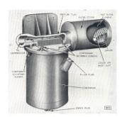
Fig. 4. Combined air filter and anti-freezer.
