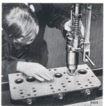
Fig. 30. Grinding valve seats.
