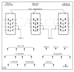
Fig. 31. Diagram of 18 way relay operated switch panel.
