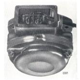
Fig. 72. Engine speed indicator generator—with cover removed.
