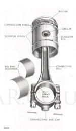
Fig. 42. Piston and connecting rod assembly.
