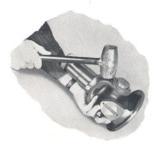
Fig. 4. Method of removing needle roller bearings from universal joint.
