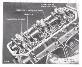
Fig. 62. Injectors and leak-off pipes in position in cylinder head.
