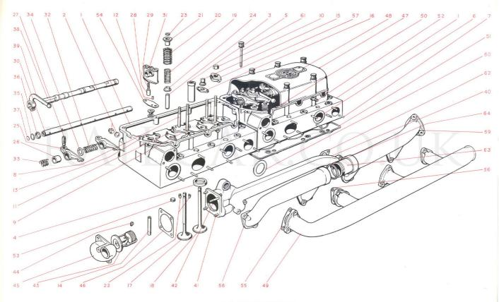
Fig. 33. Exploded view of cylinder head.
