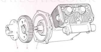
Fig. 90. The air compressor.
