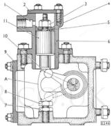
Section through throttle control motor showing travel of actuating lever at full throttle.
