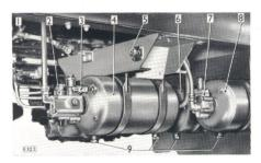
Fig. 5. Air reservoirs, unloader and diverter valves.
