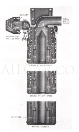
Fig. 93. Operation of the oil-bath air cleaner.
