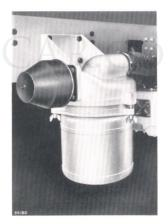
Fig. 92. The engine air cleaner.
