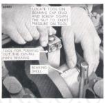
Fig. 48. Removal of main bearing shell.
