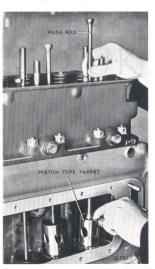
Fig. 36. Removing push rod and tappet (engine in stand).
