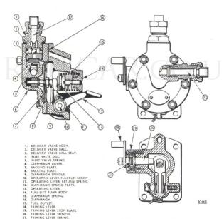
Fig. 42. Sections through C.A.V. fuel-lift pump.
