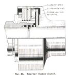
rig. 86. Starter motor clutch.
