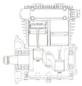
Fig. 91. Sectioned view of air compressor.
