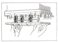
Fig. 10. Removing the Cover Plate (1st, 2nd and 3rd Speeds).
