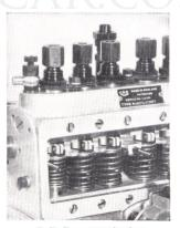
Fig. 78. The pump control quadrants.
