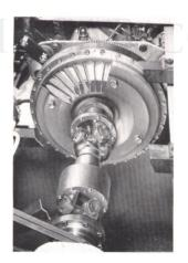
Fig. 4. Fluid coupling in position, shown part cut away.
