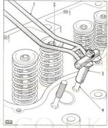
Fig. 10. Removal of valve springs.
