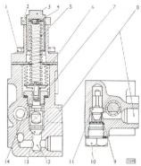
Fig. 9. Sectioned view of diverter valve.
