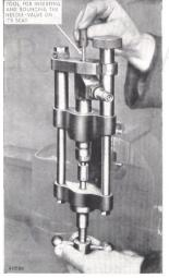
Fig. 67. Clamping the nozzle after centralizing the needle valve.
