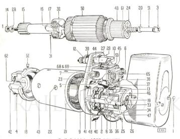
Fig. 63. Exploded view of C.A.V. starter motor.
