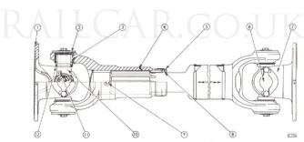
Fig. 2. Universal joint with tubular shaft.
