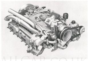
Fig. 4. Front right-hand view of the R/E.680 engine.
