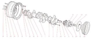
Fig. 54. Exploded view of crankshaft.
