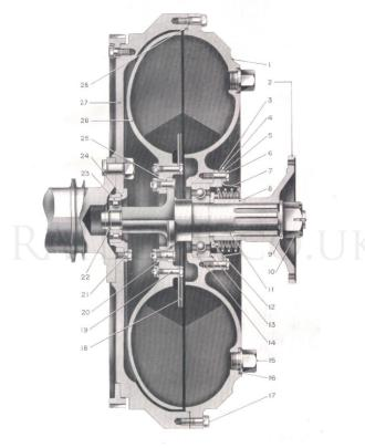
Fig. I. Section through fluid coupling (L-type).
