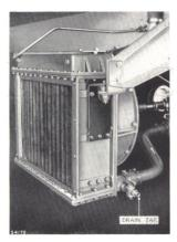
Fig. I. Radiator showing position of drain tap.
