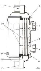
Fig. 51. Section through oil cooler.
