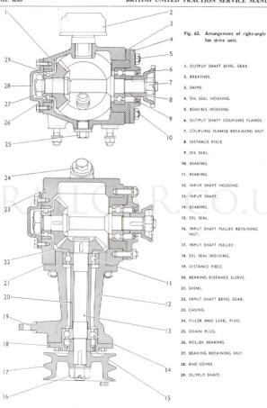
Remove the nuts and washers and withdraw the input shaft and housing assembly; retain the shims fitted between the housing and the casing.
