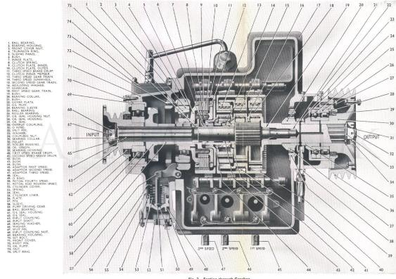
Fig. 2. Section through Gearbox.
