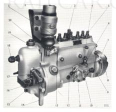
Fig. 36. Fuel-injection pump.
