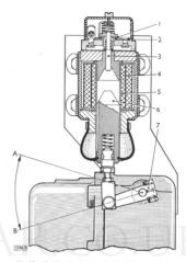
Fig. 30. Section through engine shut-down solenoid.
