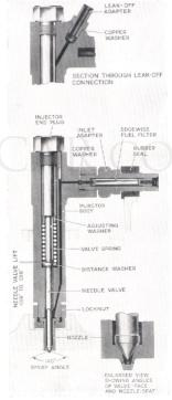
Fig. 63. The injector unit.
