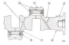
Fig. 17. Diagram of crankshaft oil passages.
