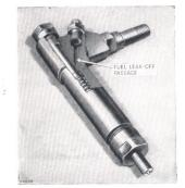
Fig. 66. Part sectioned view of injector unit.
