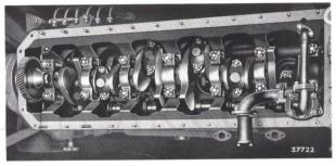
Fig. 45. Crankshaft in position.
