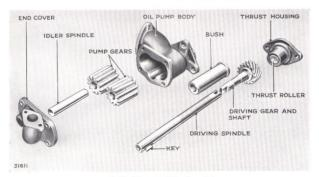
Fig. 13. Oil pump and drive dismantled.
