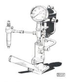
Fig. 25. C.A.V. hand-testing pump for injectors.
