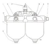
Fig. 43. Arrangement of fuel filter (C.A.V.)-twin paper element type.
