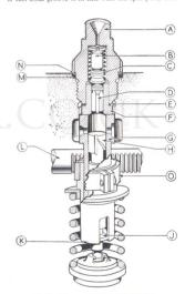
Fig. 75. The pumping element assembly.
