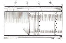
Fig. 20. Method of measuring piston ring gap.
