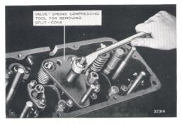
Fig. 32. Valve spring compressing tool.
