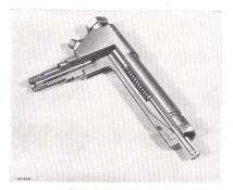
Fig. 61. An injector unit sectioned.
