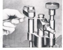
Fig. 74. Checking the needle valve lift.
