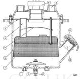
Fig. 36. Section through exhauster oil reservoir.
