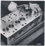
Fig. 31. Test gas-tightness of valve on its seat.
