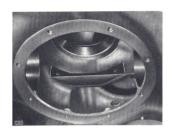
Fig. 6. Final drive casing showing oil trough.
