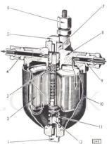
Fig. 44. Section of fuel filter (C.A.V.)-paper element
