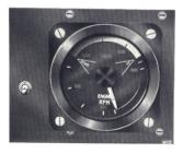
Fig. 26. Engine speed indicator and switch.
