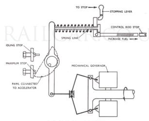
Fig. 80. Principle of the mechanical governor.
