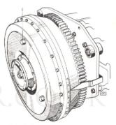
Fig. 37. Position of engine flywheel for fuel-injection pump spill cut-off point and (1) for filling or topping-up.
