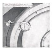
Fig. 53. Checking flywheel for running true.
