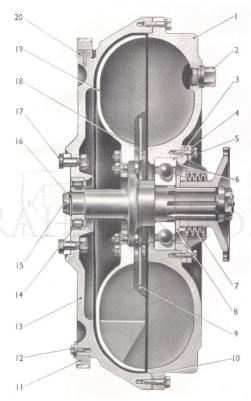
Fig. 2. Section through fluid coupling (A - type).
