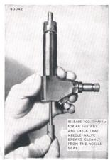
Fig. 72. The inverted test.
