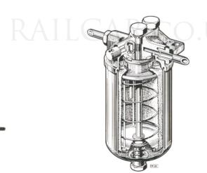
Fig. 82. Fuel filter (cloth element)
