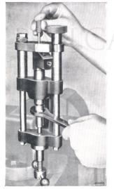
Fig.\$71. Tightening the nozzle clamp nut.
