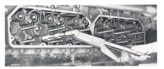
Fig. 23. Tightening head nuts with torison spanner.
