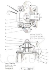
Fig. 85. Solenoid switch.
