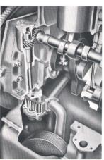
Fig. 15. Oil pump drive from camshaft (engine in stand).
