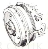
Fig. 13. Position of the flywheel for inlet valve opening.
