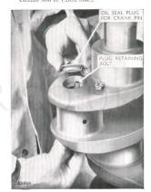
Fig. 50. Removal of oil seal plug.
