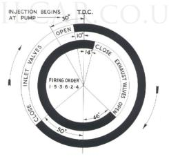
Fig. 6. Valve timing diagram.
