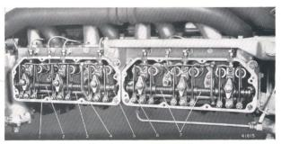
Fig. 22. Cylinder heads in position showing valve gear.
