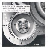
Fig. 38. Camshaft timing marks.
