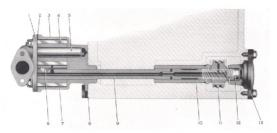
Fig. 12. Plan view of oil pump and drive
