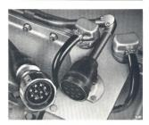
Fig. 27. Engine plug and socket.
