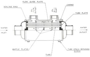
Fig. 19. Sectioned view of oil cooler.
