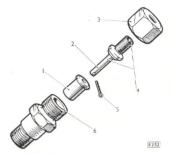
Fig. 46. Exploded view of air release valve.
