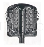
Fig. 21. Engine crankcase breather.
