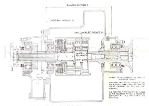
Fig 22. Method of Determining Thickness of Adjusting Washer.
