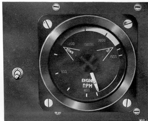
Fig. 26. Engine speed indicator and switch
