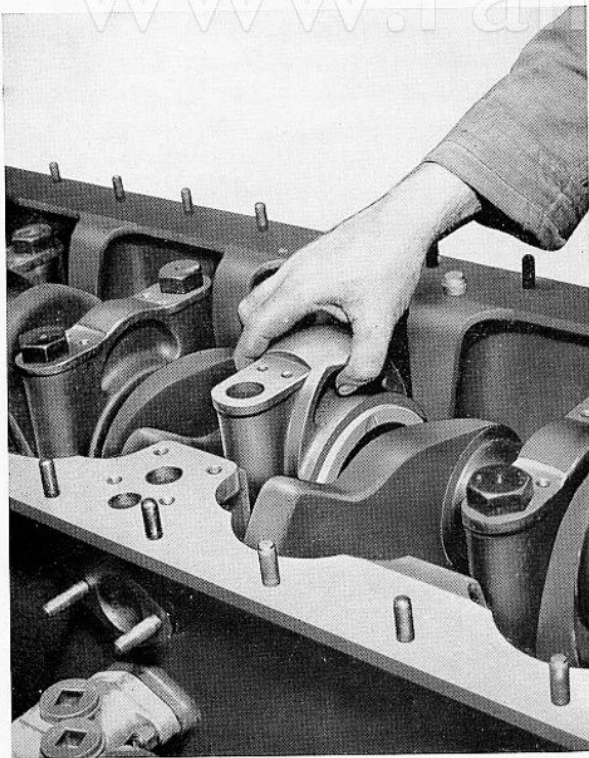
FIG. 4. REMOVING BEARING CAPS
