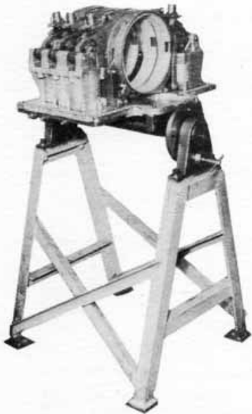
Fig. 20. Gearbox assembly stand with baseplate and brake-band gear in position.
