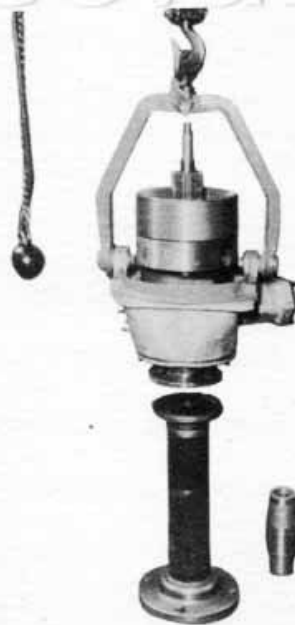
Fig. 21. Special equipment used for assembly of gearbox running gear.
