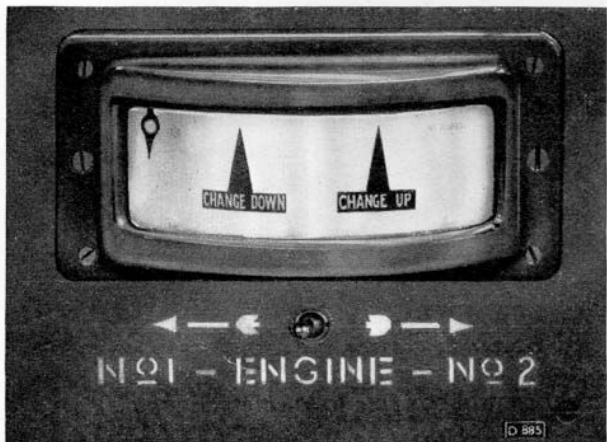
Fig. 28. Engine speed indicator and switch (belt driven generator type).
