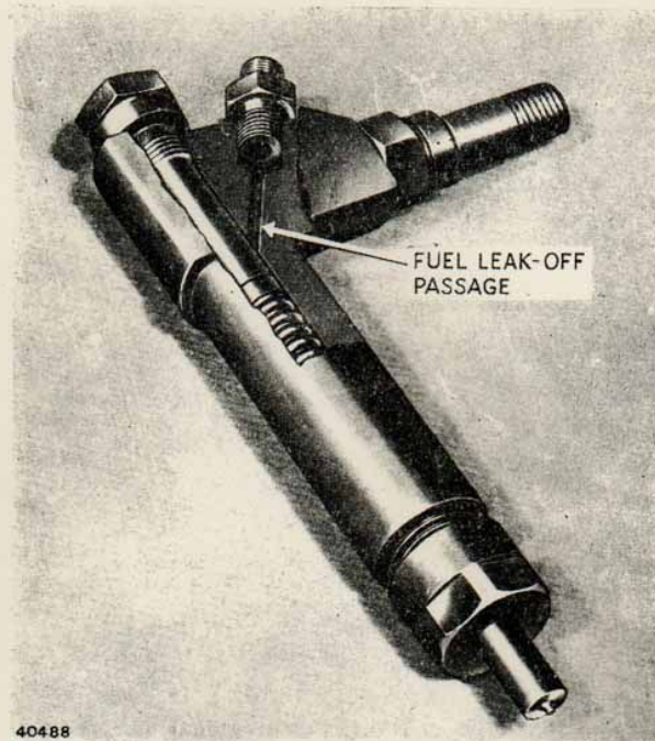
FIG. 49. PART SECTIONED VIEW OF INJECTOR UNIT.
