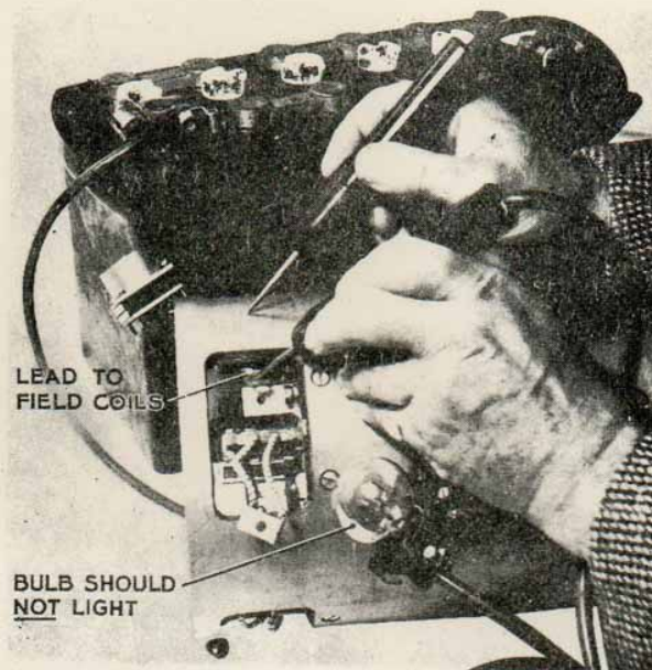
FIG. 7. TESTING FIELD COIL FOR EARTH.
