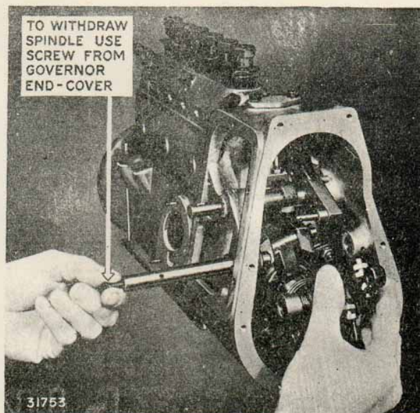
FIG. 44. REMOVING LINKAGE SPINDLE.
