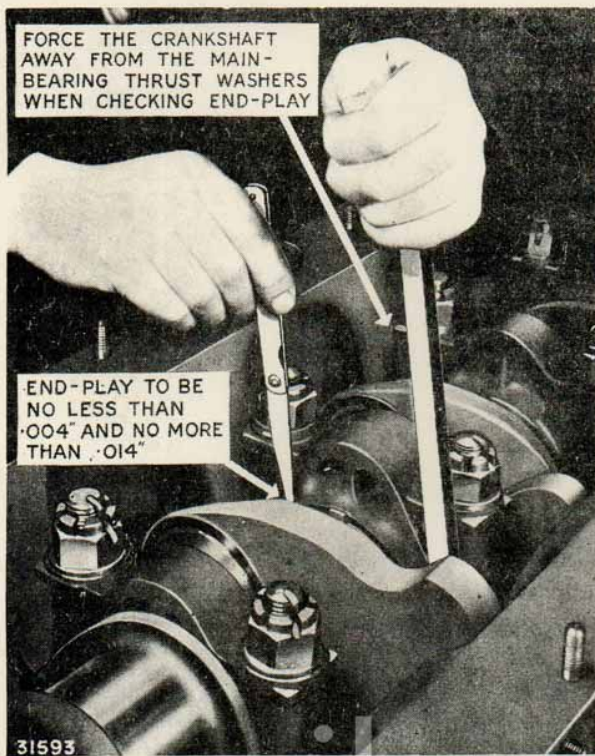
FIG. 77. CHECKING CRANKSHAFT END - PLAY.
