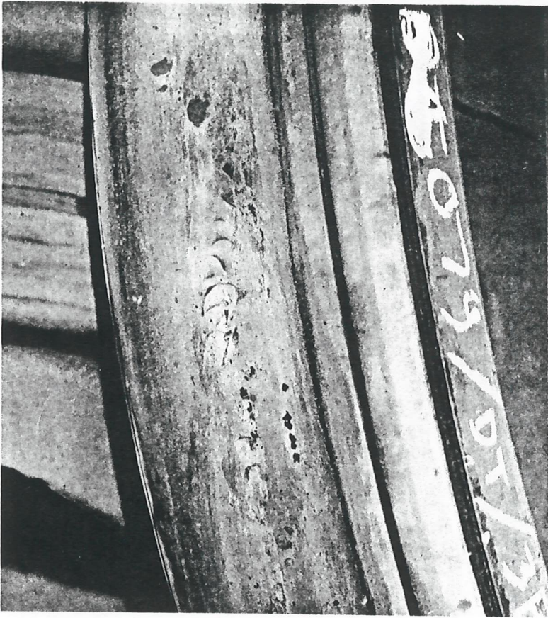
FIG. 2. High Speed Wheelslide Damage.
