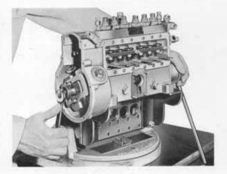
Fig. 8. Removing the governor
