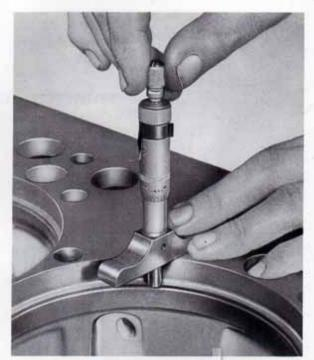
Fig. 2 Measuring distance from crankcase face
