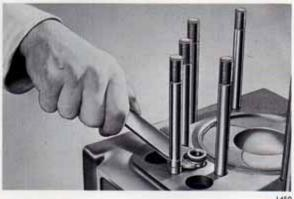
Fig. 6 Removing the transfer bobbins
