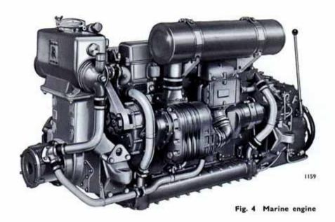
The crankshaft is nitride hardened and has at the front end an externally mounted viscous damper, which reduces the crankshaft oscillations at all speeds. A pinion on the crankshaft drives the timing gears from which are driven the fuel injection pump and the camshaft.
