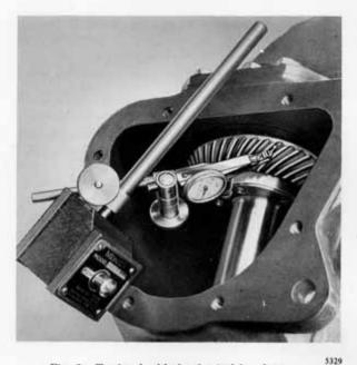
Fig. 2 Testing backlash of spiral bevel gears
