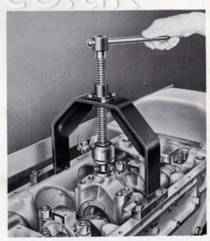
Fig. 4 Removing main bearing cap
