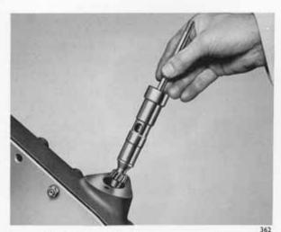
Fig. 14 Removing the service counter drive
