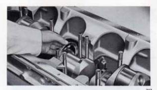
Fig. 8 Fitting the upper half thrust washer
