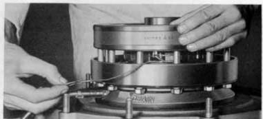
Fig. 55 Fitting freewheel outer race
