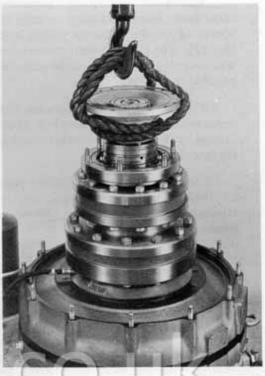
Fig. 24 Removing freewheel assembly
