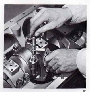
Fig. 6 Measuring a big end bolt for stretch
