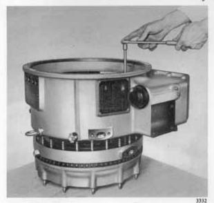
Fig. 31 Using extractor screws to separate clutch and turbine housing
