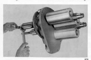
Fig. 10 Fitting rotors to drive end plate
