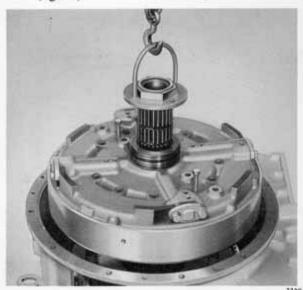
Fig. 29 Lifting clutch carrier assembly
