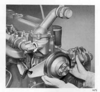
Fig. 5 Removing the coolant pump
