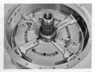
Fig. 28 Extractor screws in position for withdrawing clutch carrier
