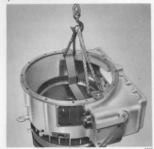
Fig. 32 Attachment of sling for lifting clutch housing
