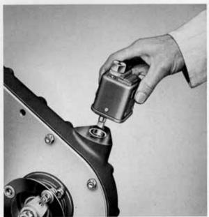
Fig. 13 Removing the service counter
