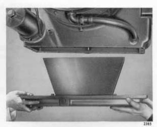
Fig. 5 Removing clutch sump cover
