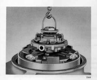
Fig. 51 Lowering clutch carrier assembly into position
