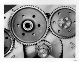
Fig. 10 Typical timing marks
