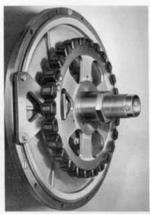
Fig. 56 Drive spider assembly tool in position
