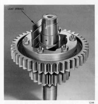
Fig. 14 Position of leaf springs for fitting
