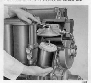
Fig. 14 Removing main filter bowl
