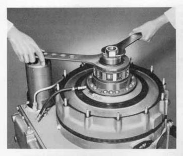
Fig. 23 Removing freewheel forward cage and cam
