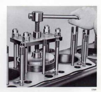
Fig. 4 Replacing a cylinder liner
