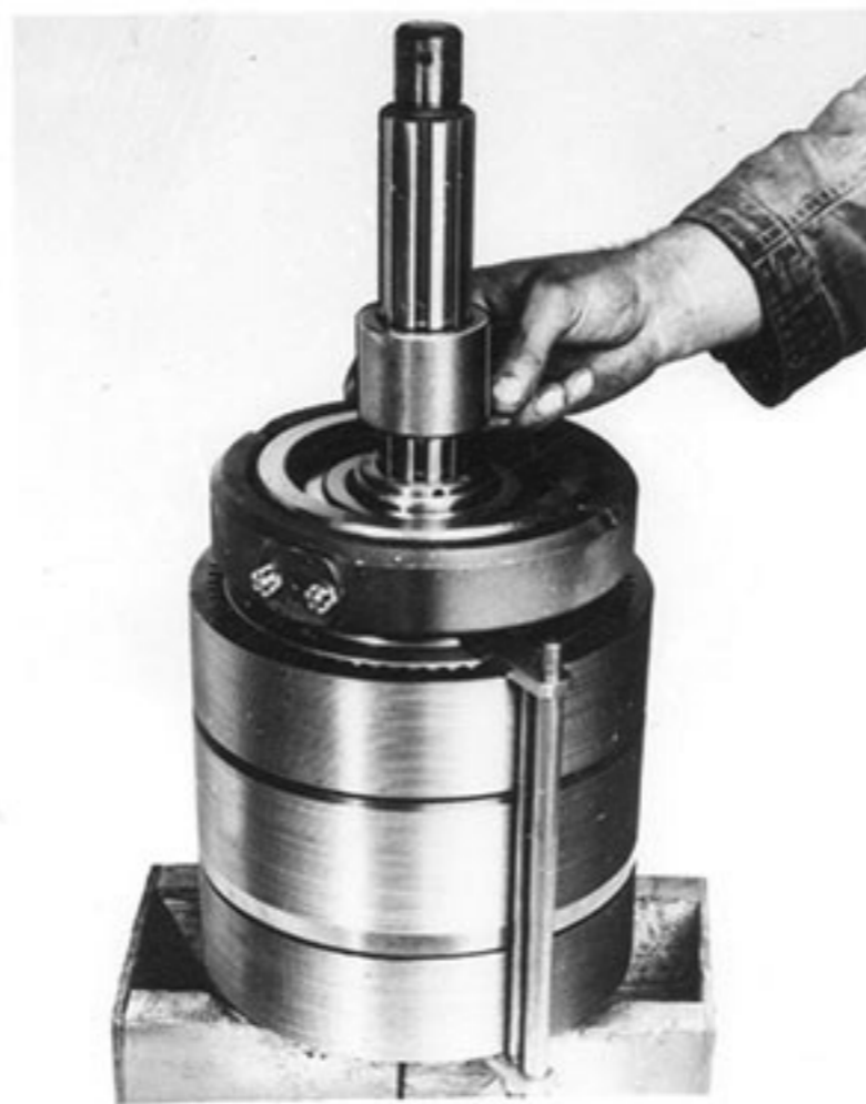
23. THE SLEEVE IS FITTED.
