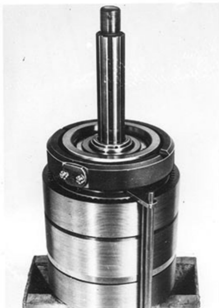
22. THE CLAMP IS FITTED TO THE RUNNING GEAR AND THE TRUNNION RING ASSEMBLY IS FITTED.
