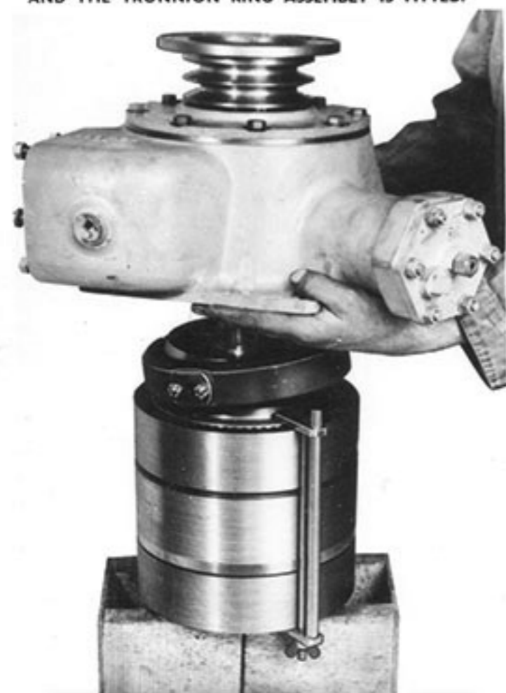
25. FIT THE ASSEMBLED FRONT COVER TO THE RUNNING GEAR.
