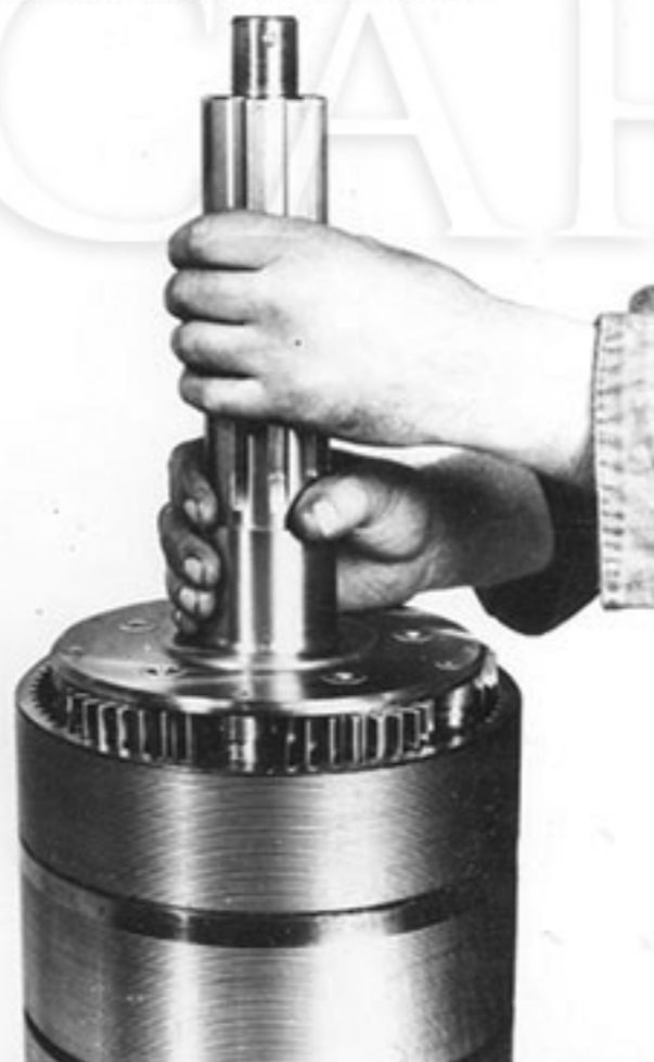
29. THEN FIT THE OUTPUT SHAFT.
