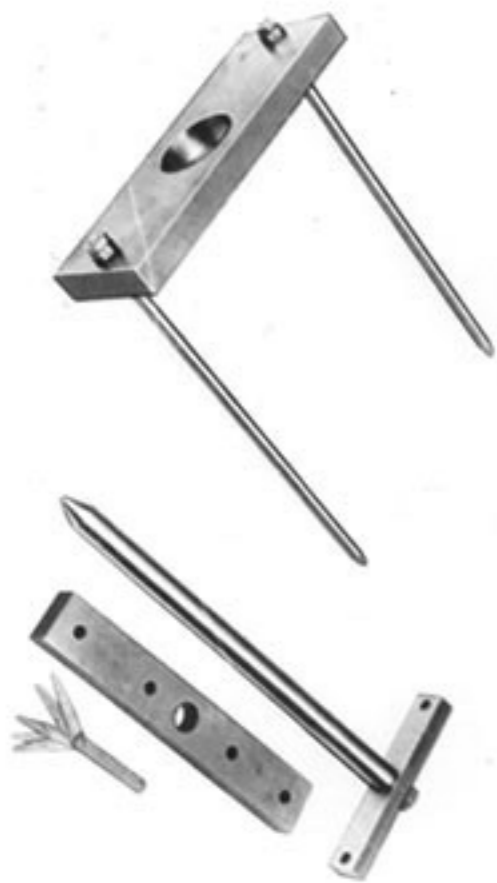
1. APPARATUS USED FOR MEASURING LENGTH OF GEARCASE AND RUNNING GEAR.
