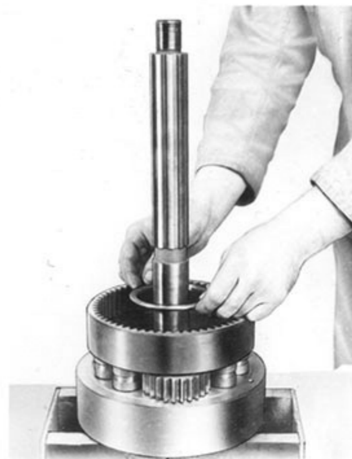
15. 1ST. SPEED DRUM IS THEN POSITIONED AND BUSH IS FITTED.
