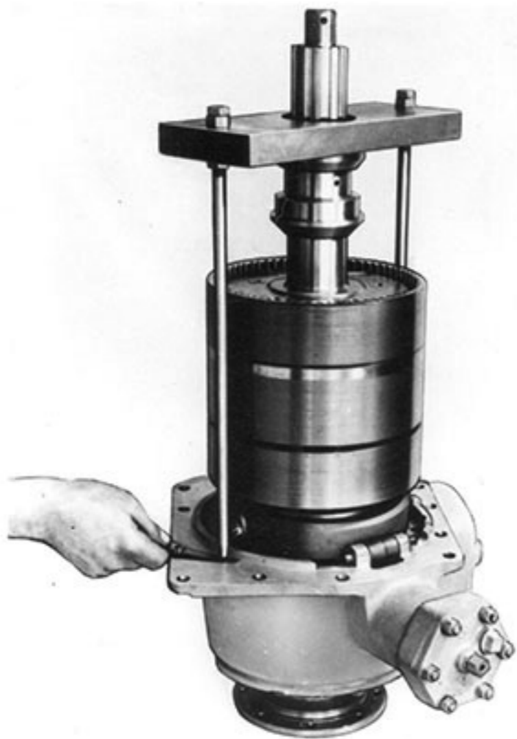
31. MEASURE THE LENGTH OF THE RUNNING GEAR.
