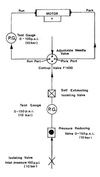
FIG 8 - Test Rig - Equipment and Piping Arrangement
