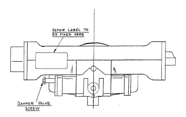
FIG 10 - Motor - Label Postion
