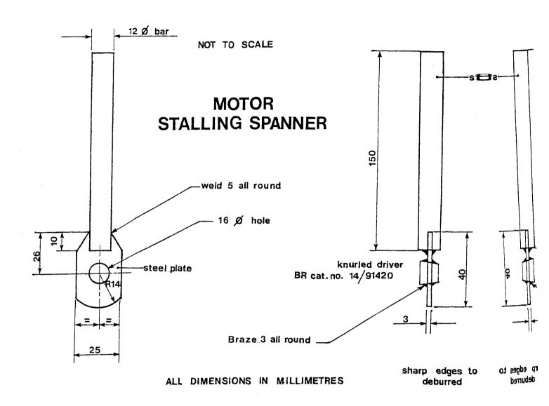
FIG 9 - Motor Stalling Spanner
