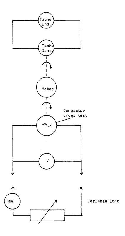
Figure 3. Generator Test Rig
