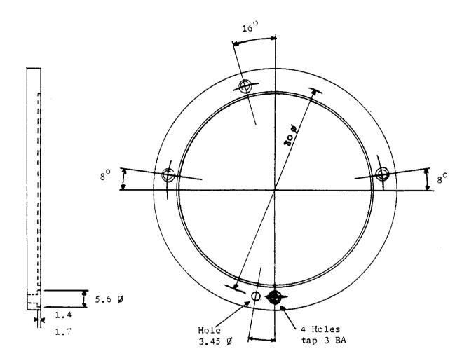
Figure 1. RE3340 Generators: Magnetic Shunt with Four Grub Screw Positions
