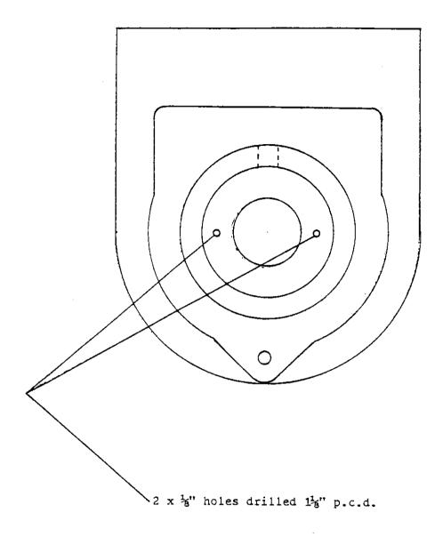
Figure 2. AEI Type JB Generators: Holes for Drive End Bearing Removal
